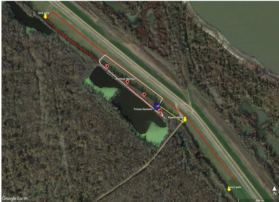
Figure 3. Proposed configuration for the installation of fiber optics, Black Hawk, LA.
