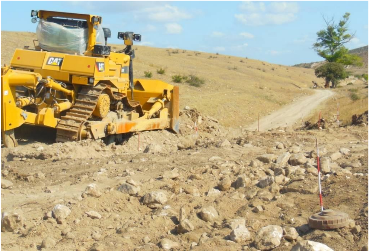
Above: Base Metals' tractor on the Janatagh road where it struck a minimum metal anti-tank mine. In the front, right of the picture is another plastic AT mine that HALO's mechanical clearance team found during its clearance. This second mine was also fused and armed – a fatal accident waiting to happen.
