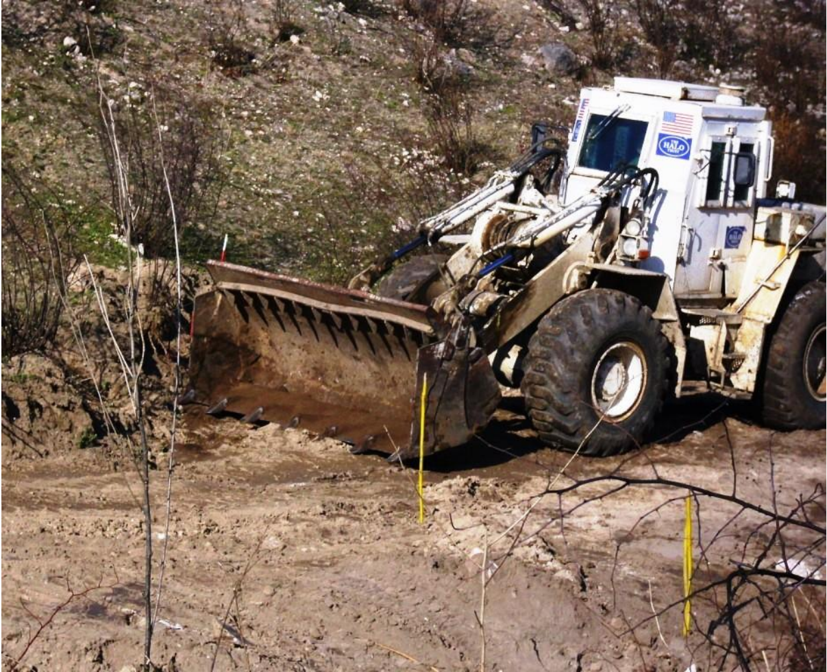
Above: HALO's USAID funded mechanical team clearing in Berdashen, 2012. The yellow sticks mark where anti-personnel mines were found and destroyed.
